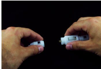
Figure 2: A user stacking input modules to create a customized digital pen.
